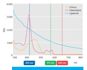
By performing premeasurement photometry on the initial bolus, the system can display hemolysis, icterus and lipemia status as a flag. The laboratory can set thresholds for each flag and measurement parameter.
